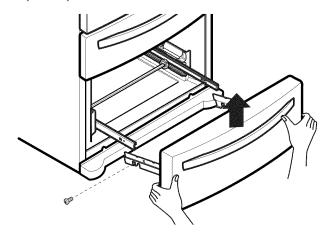
**4.** With both hands, flex the center bar enough to allow the gears on both ends to release from the track.
